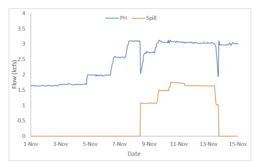
Figure 14. Hourly Flows PWR vs. Spill (Big Cliff Dam).
